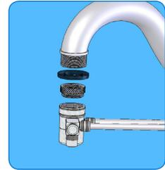
Diverter Valve Attachment with adapter
